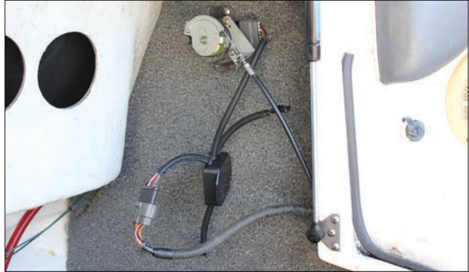
Step 3 Connect the corresponding STBD or PORT throttle node to the APS, ensuring that the connector latch is engaged. Connect the throttle node to the wiring harness, ensuring that the connector latch is engaged.
