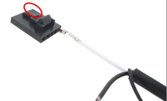
Figure 15-3: Position the white wire just inside the slot on right, denoted by the small arrow (in circle above). The small “retention clip” of the contact should be oriented downwards.
